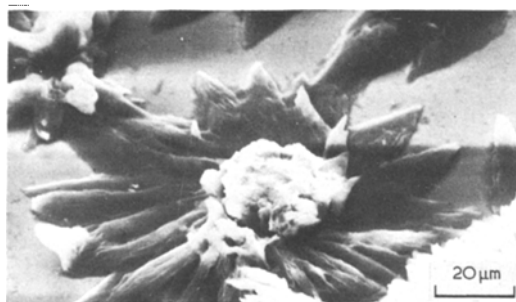
Figure 4 Scanning electron micrograph showing oxide nuclei on (111) surface of InP following anodization in PGT, pH = 9.4, at a current density of 0.16 \text{ mA cm}^{-2} .
